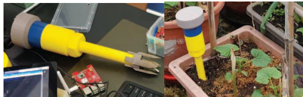
Figure 4. Data Collection Agent Sensing Device (include LoRa Mini +YL69+ DS18B20)
